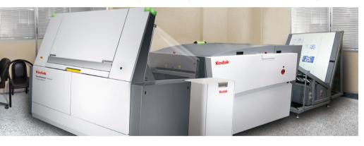
Imak Offset like many other advanced printing houses uses the direct computer-to-plate exposure. This technology ensures the minimum colour quality loss during the image transfer. This process involves CIP4 protocol that transfers technical values of the image to the control panel of the print machine and the machine performs all necessary colour adjustments automatically.
